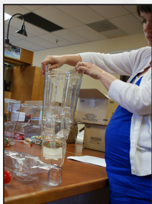
6.Remove Band Take 2 sides of bin body apart and remove rubber lip seal. Replace with polycarbonate lip seal (see inset right, #19).
