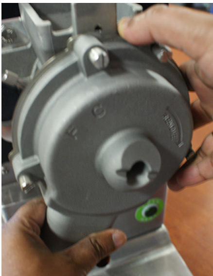
Rotate Cover clockwise to unlock Pull out once aligned with slots.
