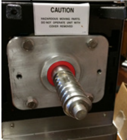
Wipe the auger, rotary seal and housing mounting plate thoroughly using a dry cloth
