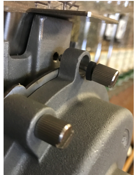
Loosen anti rotational screw until it is as shown here.
