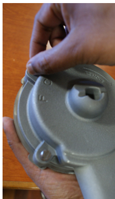
Wipe the auger, rotary seal and housing mounting plate thoroughly using a dry cloth
