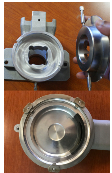
Wipe thoroughly internal and external surfaces of the hopper, shutter and pins using a dry cloth
