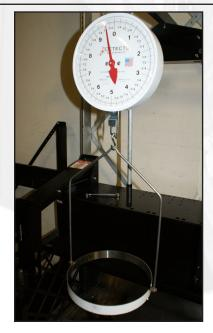
13. Attach Yoke Attach the scale hanging yoke on "S" hook at location shown.
