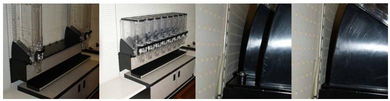
6.Step and Repeat and Install the Bins Once the retainer buttons have been correctly installed on the top shelf part, begin installing the gravity bins across this top shelf.
