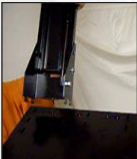
4. Install the Swing Down Arm Once you have inserted the swing down arm into the slotted holes in the top shelf, use both hands and slide the arm assembly back to lock the arm in place.
