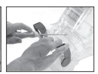
Increasing the Food Flow Disengage travel stop tab with a screwdriver and simultaneously drive the travel stop toward you by pulling down on the dispensing handle.
